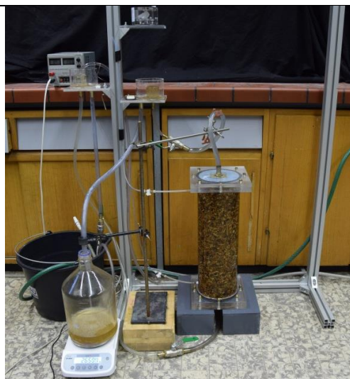
Column (8,7 L) for characterization of woodchips properties
