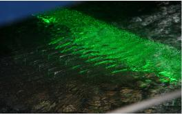
Figure 1: Left: Schematic of Particle Image Velocimetry setup. Right: A model of vegetation patch (e.g. group of glass blades) in a water flume illuminated by laser sheet for Particle Image Velocimetry.
