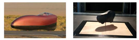
Figure: Velomobile on speed record run and scaled model velomobile in wind tunnel test.
